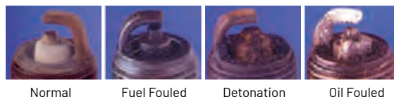
Spark Plug Diagnosis Pictures Courtesy Of Autolite
