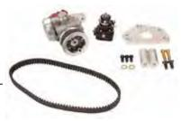
Complete assembly weighs just over 5 lbs., includes power steering pump with Sweet-designed Waterman fuel pump, 33-tooth HTD pulley, 800mm x 20mm wide HTD drive belt, aluminum cylinder head mount, and Aeromotive dual-adjustable fuel pressure regulator. System is compatible with alcohol or gasoline.
