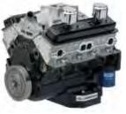
aluminum intake manifold. Carburetor, starter, ignition, plug wires, water pump, distributor, and exhaust not included. **Note: Requires an externally balanced flywheel/flexplate. Distributor with melonized gear must be used on engines with steel camshafts, or engine damage will occur.**
