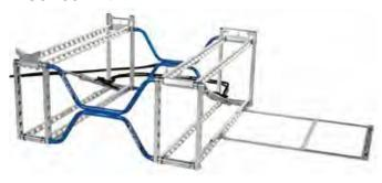
Engineered exclusively for dirt modifieds or dirt late models, topof-the-line, machined aluminum lift eases repairs or setup changes between races, virtually eliminating the need for traditional pit jacks and jack stands. X-Series lift is 20" wide in the rear and 18" in the front with 1.625" bolt-on right front risers, and utilizes a dual action, 12-volt powered 2,300 PSI hydraulic pump with Sweet Manufacturing cylinders. Lift is sold complete with hydraulic pump and hose kit.
