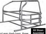
halo, windshield posts, front and rear dash bars, three door bars for the left side, and a Z-bar for the right side. Also included are two lengths of 1-3/4" tubing to weld to the factory pinch welds and two lengths of 1-1/2" tubing to connect the two sides, creating a solid foundation for the cage and seat mount.
