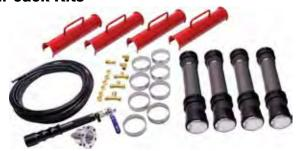
The air jack system fastens directly to your chassis and uses air pressure supplied by a nitrogen tank to raise your entire car in seconds! Kits include four air jack cylinders with a 11.75" or 15.25" stroke length, cylinder mounting rings, air coupling with receiver, installation kit, safety stands, and detailed instructions. Air jack kits have a 3000-lb. capacity. Note: A nitrogen tank, high-pressure regulator, and an air hose rated at a minimum of 400 PSI is required for operation.
