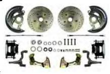
powder-coated calipers, stainless brake hoses, backing plates, caliper brackets, and required hardware.
