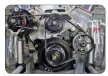
power steering pump with bolt-on tank, Denso 138mm heavy-duty alternator, CNC-machined pulleys and brackets, belts, and necessary hardware.
