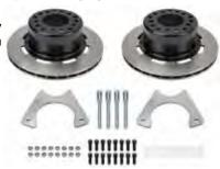
with flanges larger than 5-3/4" must use cast aluminum rotor hats, ALL42128 or ALL42129. Kit includes rotors (.810" x 11.75"), universal rotor hats, rotor bolt kits, caliper mounting bolts, and caliper mounting brackets for GM intermediate metric-style calipers (ALL42083 and ALL42084). **Note: kit does not have provisions for parking brake.**
