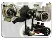
pulleys, mini alternator with bracket, aluminum power steering pump with integral reservoir and bracket, Edelbrock water pump, drive hub, belt guides, drive belts, and all hardware.
