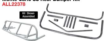
Kit includes pre-bent and notched 1-3/4" x 0.095" wall tubing to assemble a strong rear bumper that can be mounted to any width chassis and support the Allstar Performance and other aftermarket 1983-88 Monte Carlo SS rear bumper covers. Kit must be welded.
