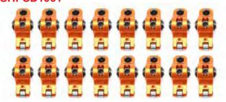
Identical to traditional Sharp rocker arms but profiled to reduce valvetrain mass, while providing increased valve spring, stud girdle, and valve cover clearance. Sold in a set of 16, rockers have a 1.5:1 ratio and are designed for use with 3/8" studs. Fits all 1955-99 small block Chevy.
