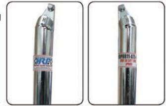
These revised posts have a clear recognizable proprietary "approved" decal along with a stamped "H". These revised posts will be the only HRP manufactured top wing post sold.
