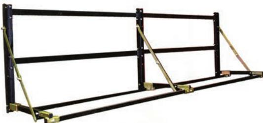
Unique heavy-duty steel rack mounts on 16" centers and adjusts from 18" to 26" for different tire diameters. Quickly unfolds from the wall and adjusts to full length. Removable lock pins allow easy storage.
