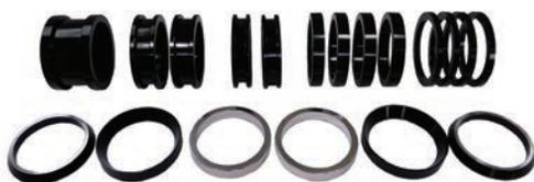
19-piece billet aluminum spacer kit contains all spacers needed to do both sides of the axle. Contents of the kit include (4) 1/4" spacers, (4) 1/2" spacers, (2) bearing shoulders, (2) inner cones, (2) outer cones, (2) 3/4" lightened spacers, (2) 1" lightened spacers, and (1) 2" lightened spacer.
