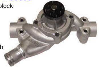
Pump is 5.825" high, with a heavy-duty 3/4" shaft, 1/2" billet steel hub, -16AN side outlets, and stock mounting holes.
