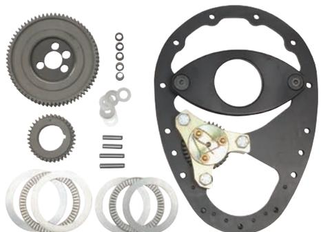
Gear drives are complete with cam, crankshaft, and idler gears; needle bearing thrust kits; offset degree bushing kit; extra-long dowel pins; and installation instructions. Gear drives are commonly used with [ALL90080](#) and [ALL90081](#) Billet Timing Covers or may be used with most stock-type covers such as the [ALL90010](#) with slight modification.
