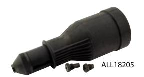
**INSTALLATION:** Always use a reversible drill and set to drill position. Experiment with high and low speeds to achieve best results. Open the drill chuck and insert the shank of ALL18205 (FIG. 1). Tighten the chuck securely and cover with "telescopic" protective sleeve. Three nosepieces are included (use the same nosepiece for 3/32" & 1/8" diameter rivets). Use the proper size nosepiece for the rivet being installed.
