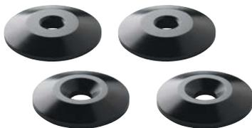
Required by NHRA for mounting funny car body to the frame structure. Black anodized 6061-T6 aluminum. 7/8" diameter. 1/8" thick. Hole for #10 screw. Two styles available: **Part No. 897100** with flat surface and **Part No. 897182** with 82° countersink for flathead screws.
