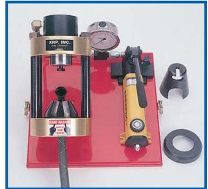
**6** Place the upper half of the crimp die over the assembly in the crimper.
