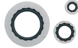
Our best sealing washer, Stat-O-Seal consists of a Buna N O-ring mechanically locked to the I.D. of an aluminum washer. When tightened, the O-ring is compressed around the bolt shank, forming a positive seal over a temperature range of -85° F to 450° F. Stat-O-Seal is more efficient than copper or fiber sealing washers.
