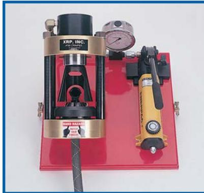
**8** Place the pusher cone into the crimp machine and pump the handle until the cone just contacts the pusher ring plate. Now, recheck! Make certain that the crimp collar is fully covered by the crimp die and the nipple has not moved.
