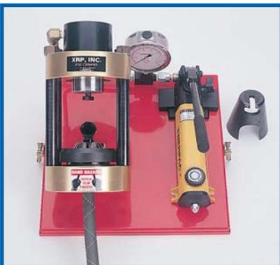
**7** Install the tapered die pusher ring plate over the crimp die. Push the plate down by hand, until the crimp die is snug on the crimp collar. Make sure the die covers the entire length of the collar.
