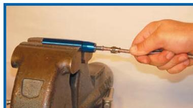
**STEP 2** Flare braid using a twisting motion.
