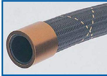
**2** Slip the crimp collar over the hose until the inside flange of the collar is against the face of the hose.
