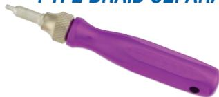
Using XRP's Separating Tool is the quickest way to flare stainless braid away from -3 and -4 PTFE hose for easy insertion of the olive during assembly.
