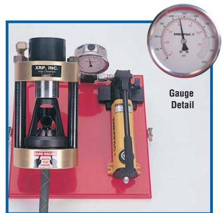
**9** Continue pumping the handle until the crimp die cage is completely closed and the pressure on the gauge indicates 4,000 to 5,000 psi. Larger sizes may require more pressure. Each die has been manufactured to provide the proper finished diameter crimp. Pressure test and inspect the finished hose assembly.
