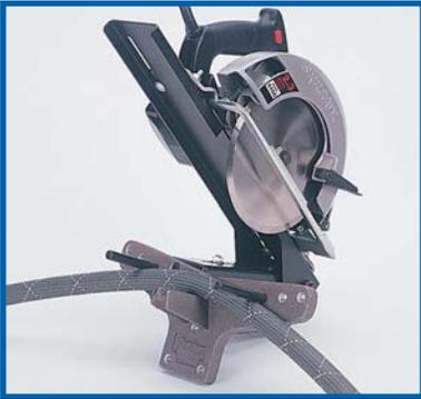
**1** Use the XRP Hose Cut-Off Blade to cut the hose to the proper length. The toothless knife edge wheel will provide a clean and square cut. May be used on stainless steel braided hose also.
