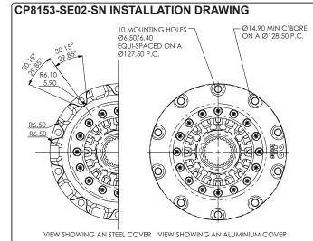
RECOMMENDED CLUTCH MOUNTING: (FOR ALL TYPES OF ASSEMBLY)
