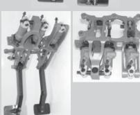
This unique pull type bulkhead mount design with master cylinders being located in the engine or front compartments allows the pushrod to remain in line eliminating all side loads making it one of the most efficient pedal box on the market. It's lightweight aluminium base, and ergonomic steel and alloy pedals offer the user the ultimate control in this critical area.
