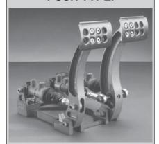
This is a general purpose floor mounted pedal box which utilises the latest high efficiency CP7854 push type master cylinders. Minimum hysteresis and balance variation are assured by the use of needle roller bearings in the centre trunnion and ball bearing pedal pivots
