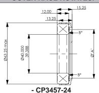
Release Fulcrum Dia 'A' = 50mm. This bearing is suitable for use with most Ø115, Ø127 & Ø140mm racing clutches.
