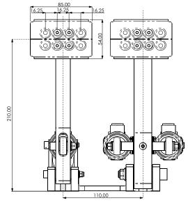
SETING UP THE BALANCE BAR ADJUST THE PUSHRODS SO THAT THE BALANCE BAR ISPERPENDICULAR TO THE PUSHRODS UNDER MAXIMUM LOAD, THE SYSTEM IS THEN SQUARE. IT IS NOT IMPORTANT THAT THE SYSTEM IS SQUARE WHEN RELEASED, BUT IT HAS TO BE UNDER LOAD.
