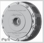
plate is fitted this will retain the diaphragm and release fulcrum and this step is omitted. Then install the main pressure plate into the clutch housing, (see pressure plate service sheet) with the raised fulcrum against the diaphragm spring and the identification mark adjacent to the similar mark on one of the clutch lugs.
