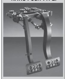
This multi ratio push type pedal box allows the pushrod to remain straight, eliminating all side loads therefore making it very efficient. The master cylinders connect directly to a high
