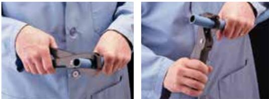
The rotating/rocking technique produces fast easy cuts.
