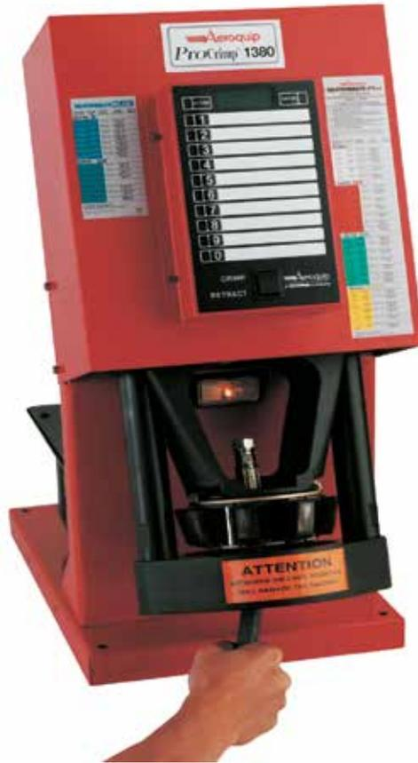
The ProCrimp® 1380 is totally compatible with Eaton's MatchMate® Plus hose assembly program. Matching and mating hose to fittings and to the tooling in the ProCrimp® 1380 make hose assembly simpler than ever. Decals have been prepared to fit the ProCrimp® 1380 with all of the MatchMate Plus hose styles, including MatchMate BLUE®.
