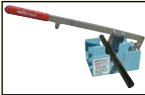
**Step 1.** Cut hose square to length with Aeroquip Performance Products Cut Off Tool (FT1258) or similar cutting device.
