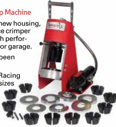
The performance version of the ET1000 builds on the success of Eaton portable crimp machines by using a 2-piece split half collet assembly in lieu of traditional one-piece die cages. The correct hose assembly crimp diameter is obtained by the use of a spacer ring that controls the stroke length of the cylinder during the crimping operation.
